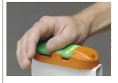
Working distance of the Emit punching unit to emit-card about 10 cm. It means that the time can unintentionally
